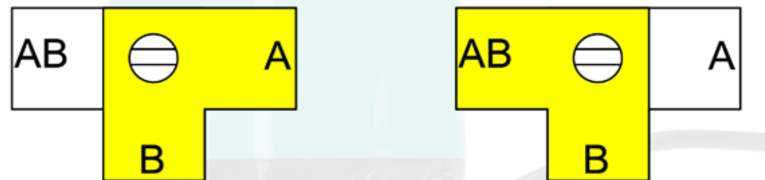
Schematic diagram of electric three-way L-type valve
